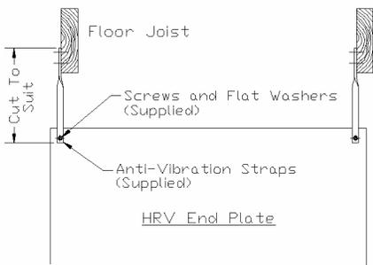
For maximum efficiency, the HRV should be installed in a heated area. The HRV is designed to be hung from the ceiling by way of the anti-vibration straps supplied. Avoid hanging the HRV directly below a bedroom or other quiet area.
