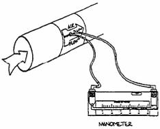
To balance the HRV, you will need a device to measure air flow. It is recommended to use either a magnehelic gauge or an air meter, both of which are available from Nu-Air. Depending on the device you are using, follow one of the two procedures below:
