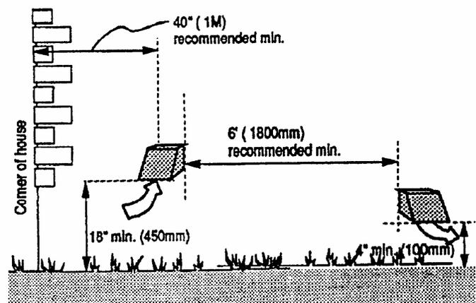
Make the insulated duct that connects the weather hoods to the HRV as short as possible to minimize airflow restrictions. Avoid sharp bends and stretch out the inner lining of the flex duct as much as possible to reduce static pressure and maximize airflow. For runs over 12', increasing flex diameter 1" to next size up will reduce pressure drop in the duct.
