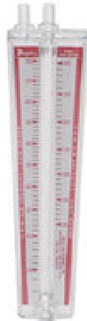
For residential applications you should have a minimum ventilation capacity of 10 cfm (5 L/s) per room. The chart that accompanies the flow grid calibrates pressure readings to airflow.
