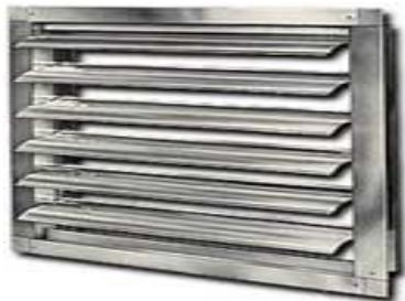
Optional gravity dampers for exhaust air and motorized intake air dampers prevent unwanted outside air from entering the space when the heat recovery unit is not operating. Factory mounted in the collar of the HRV.
